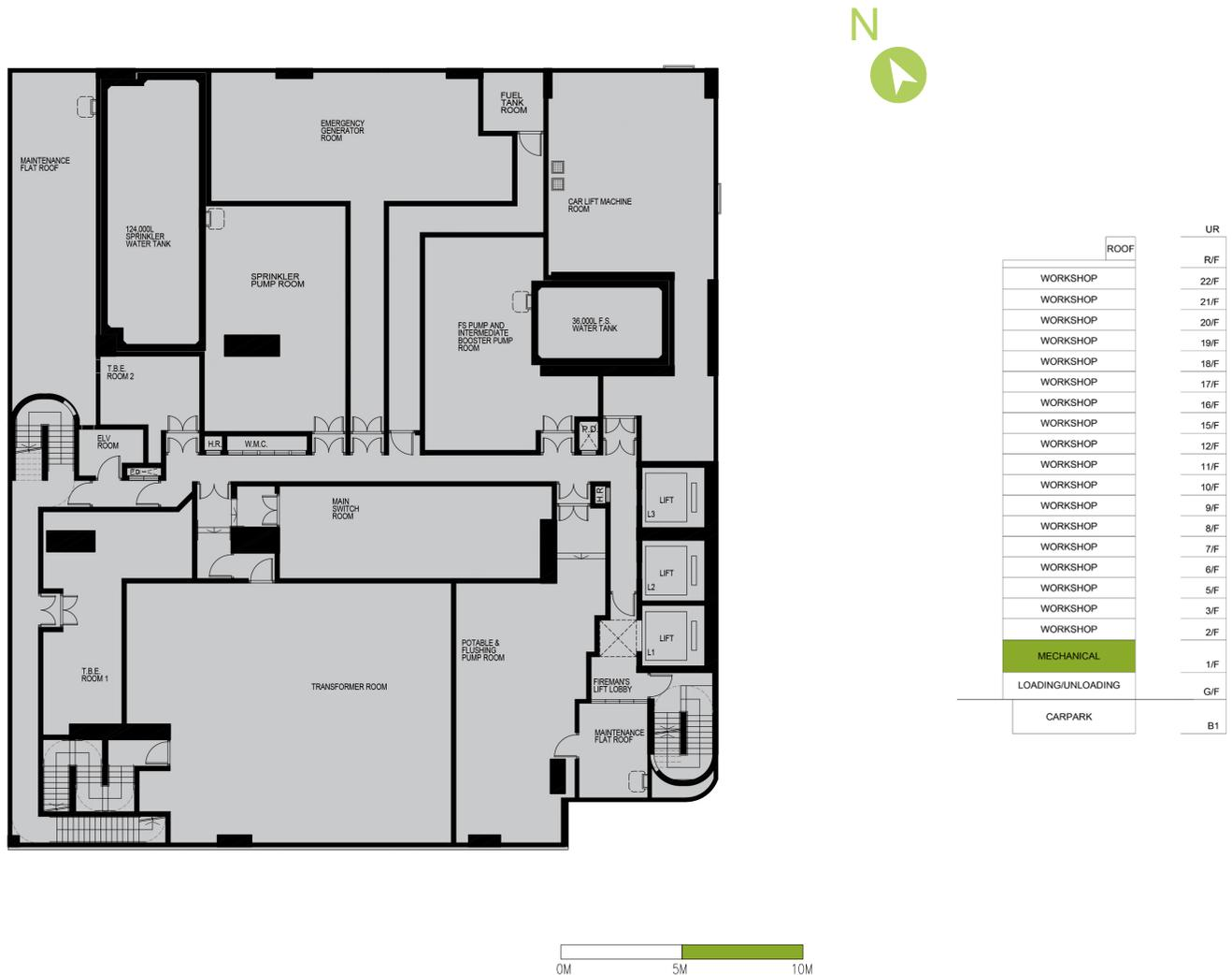
Mechanical Floor at 1/F Floor Plan
