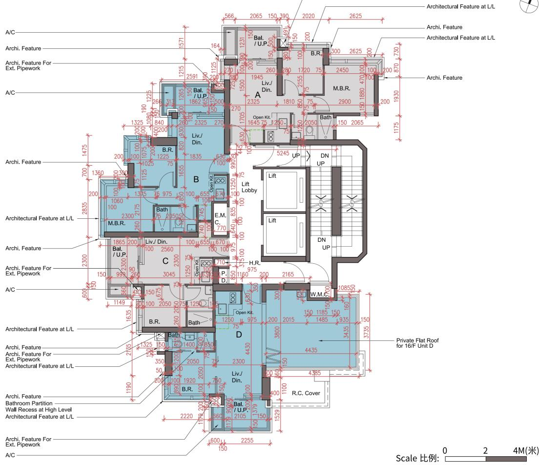
Note: The dimensions of the floor plan are all structural dimensions in millimeter.
